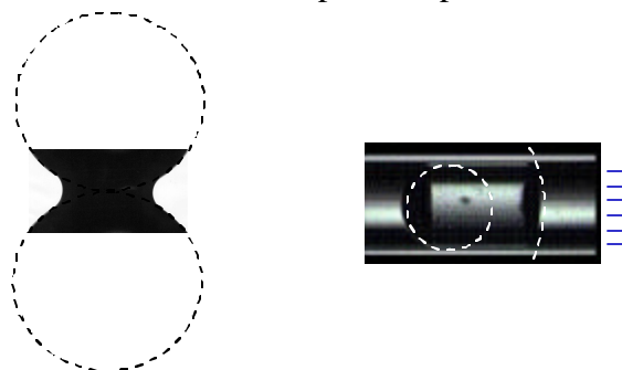
Figure 3. Mixed fluids. Microphotographs: (a) Meniscus between two 1mm diameter glass beads. (b) Water drop in 1mm capillary tube subjected to differential pressure (Alvarelos 2003) - Note that the contact angle is not constant when there are interacting menisci.
