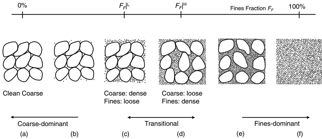
**Fig. 2.** Coarse-fine mixtures: threshold fractions; coarse-dominant, transitional, and fines-dominant mixtures; these conceptual sketches apply to gravel-sand, gravel-fines, and sand-fines mixtures
