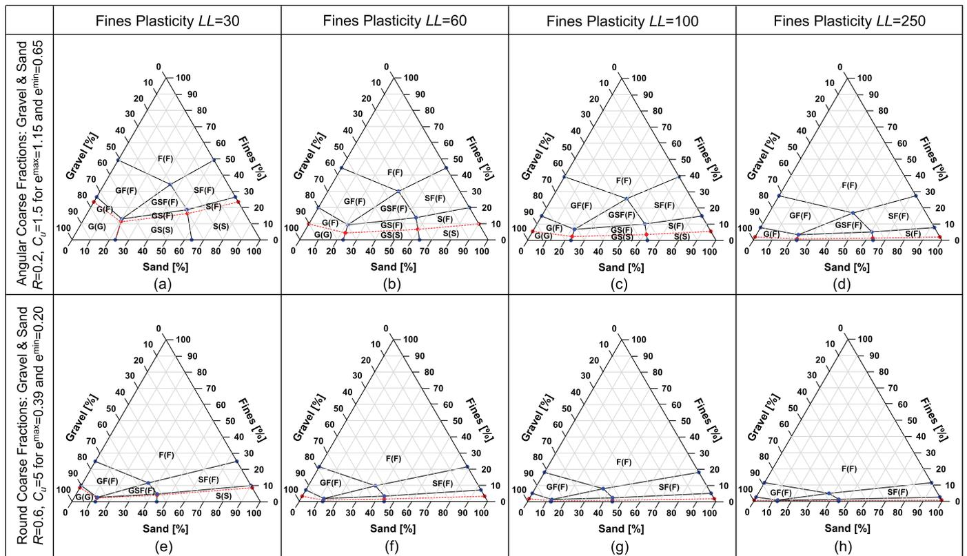
**Fig. 10.** (Color) Revised soil classification system sample charts: angular gravel and sand with (a) fines LL = 30, (b) fines LL = 60, (c) fines LL = 100, and (d) fines LL = 250; round gravel and sand with (e) fines LL = 30, (f) fines LL = 60, (g) fines LL = 100, and (h) fines LL = 250; refer to Fig. 9 for missing nomenclature in small zones
