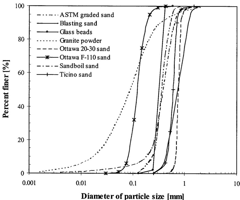
FIG. 3—Particle-size distribution for the tested soils.
