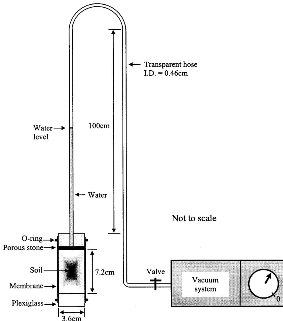
FIG. 1—Device and experimental setup used for the simple CS test.
