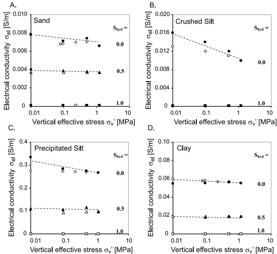
**Figure 6.** Electrical conductivity at 0.2 GHz as a function of vertical effective stress for (a) sand, (b) crushed silt, (c) precipitated silt, and (d) clay. Symbols and labels the same as in Figure 5.
