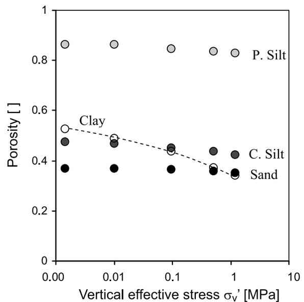
**Figure 4.** Porosity  $n$  as a function of vertical effective stress for soils saturated with deionized water. Similar trends and values are noted for soils saturated with THF solutions. The clay specimens (open circles) follow the trend denoted by the dashed line.
