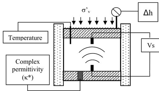
**Figure 1.** The instrumented odometer cell (zero lateral strain,  $\varepsilon_h = 0$ ) used for this study. The sample occupies the region within the cell walls.  $\Delta h$  refers to the change in height of the specimen (vertical displacement),  $V_s$  refers to shear wave velocity measured over the specimen's height, and  $\sigma'_v$  refers to the applied vertical effective stress.
