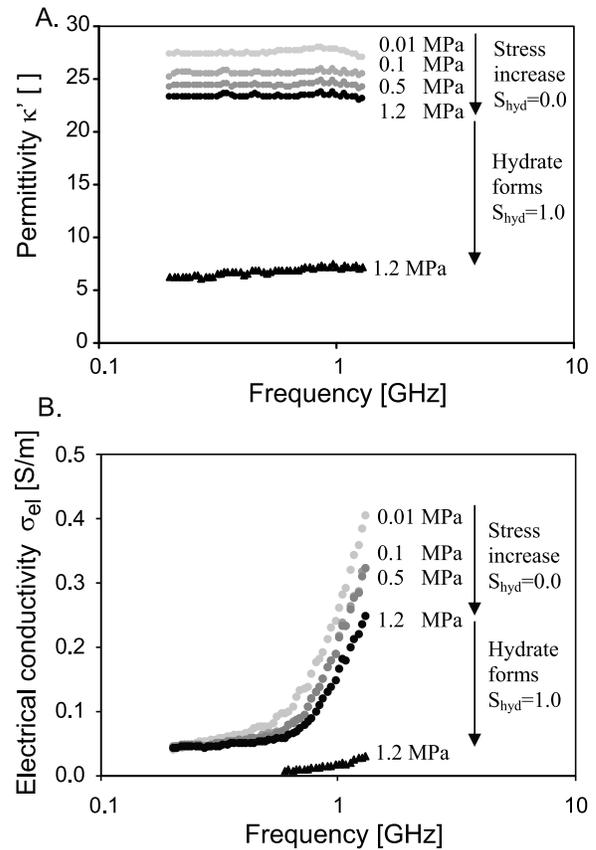
**Figure 3.** (a) Permittivity and (b) electrical conductivity spectra for different vertical effective stress levels in clay with 21% THF solution as the pore fluid. Also shown is the result obtained after hydrate formation ( $S_{hyd} = 1.0$ ) at 1.2 MPa.
