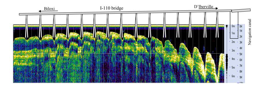
**Figure 2:** 20 kHz subbottom profiles of Bay of Biloxi Bridges. (a) Collapsed Highway 90 bridge. The profile was run approximately 1.5 m from the SE edge of the pile sets, the average separation between pile sets is 16 m. (b) I-110 Bridge. The profile was run approximately 1.5 m from the E edge of the pile sets, the average separation between pile sets is 30 m. Horizontal scales are different.
