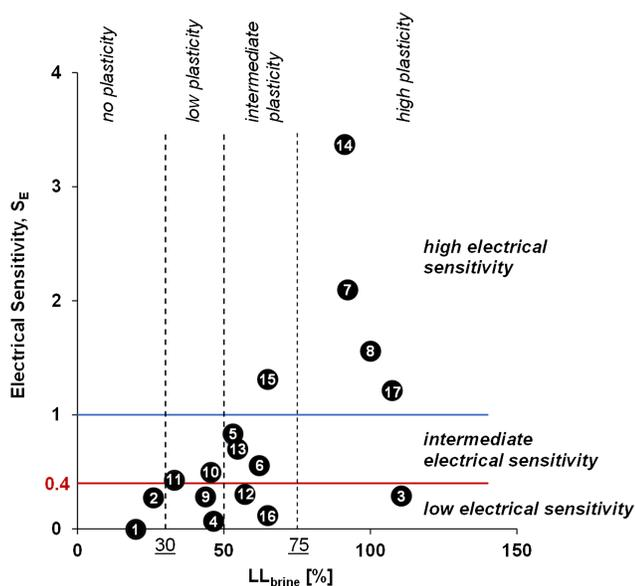
**Fig. 7.** Proposed chart for the classification of fine grains on the basis of electrical sensitivity and liquid limit; numbers in black circles refer to soils described in Fig. 4; the  $S_E = 0.4$  and  $S_E = 1.0$  lines correspond to the boundaries defined in Fig. 6
