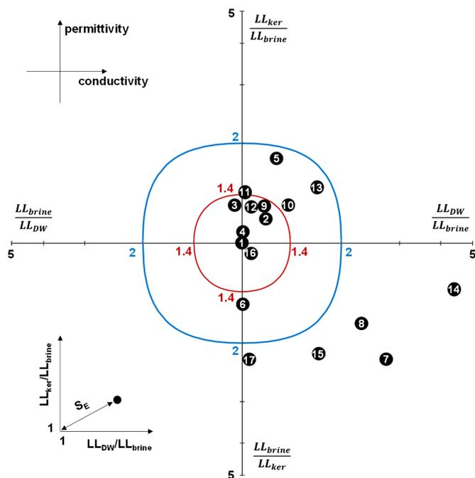
**Fig. 6.** Sediment response to changes in fluid conductivity and permittivity; values of liquid limit reported in Fig. 4 are plotted as ratios between  $LL_{DW}$  and  $LL_{brine}$  (conductivity effect) and  $LL_{brine}$  and  $LL_{ker}$  (permittivity effect); the scale changes across the origin: LL ratios are larger than 1.0 in all quadrants; the inset shows the definition of electrical sensitivity  $S_E$  [Eq. (3)]; numbers in black circles refer to soils described in Fig. 4
