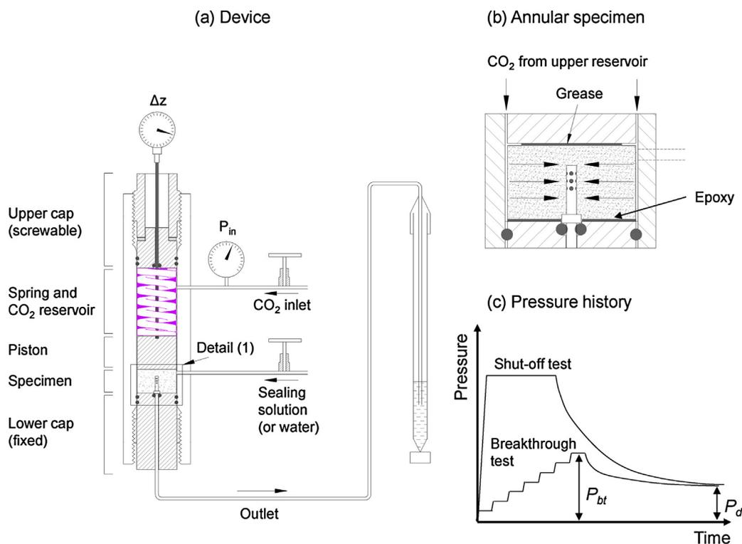
Fig. 1. Experimental device for CO<sub>2</sub>-breakthrough and sealing studies. (a) The internal spring applies a constant vertical force onto the specimen. (b) CO<sub>2</sub> infiltrates the specimen radially. (c) Pressure histories typically used for determining breakthrough  $P_{bt}$  and shut-off pressures in two different test types.
