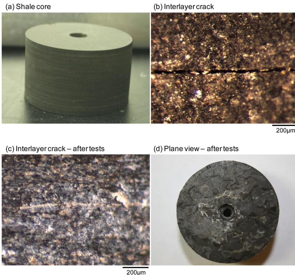
**Fig. 3.** Shale specimens. (a) Core prepared for the CO<sub>2</sub>-breakthrough test. (b) Microscopic image of interlayer crack. Post-test forensic analyses: (c) the microphotograph shows a crack filled with sub-micron bentonite particles after sealing treatments; (d) sub-micron particles deposited in the gap between cracks after sealing treatments.
