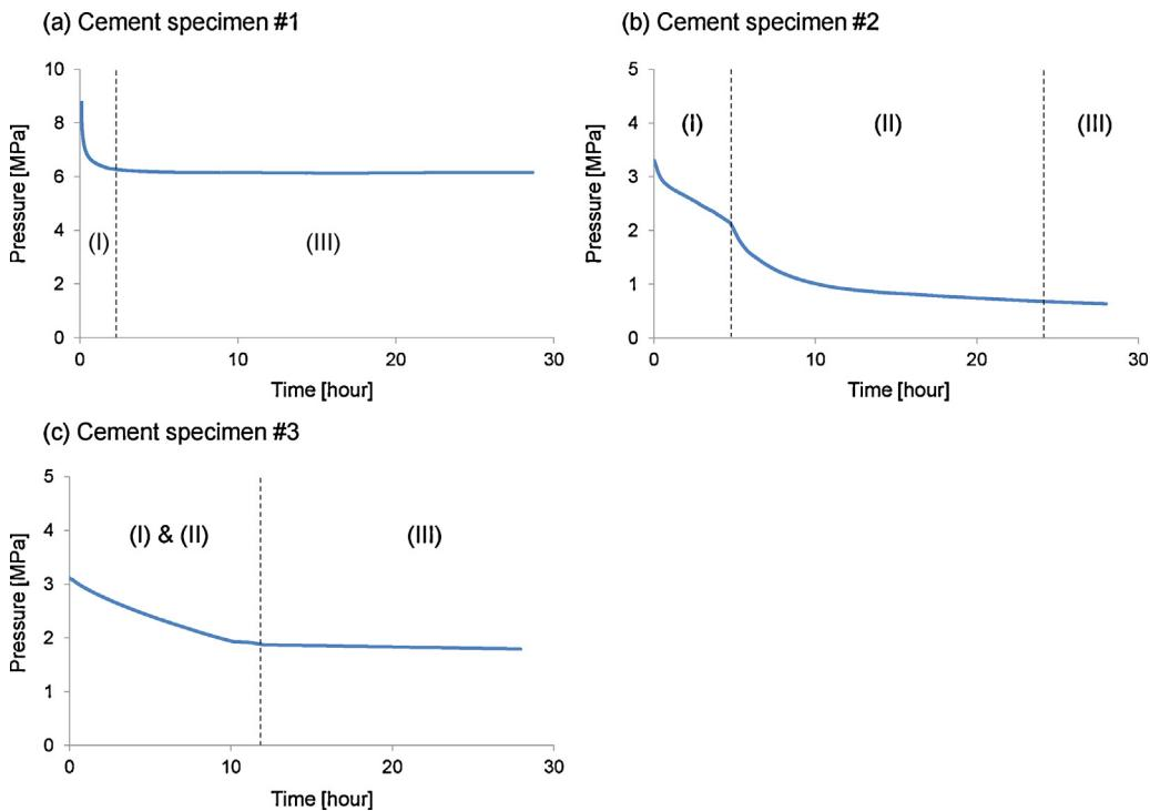
**Fig. 4.** Cement specimens – Shut-off pressures observed with three different specimens. Note: only specimen #2 exhibits a clear transition from single-phase water flow to CO<sub>2</sub> flow.
