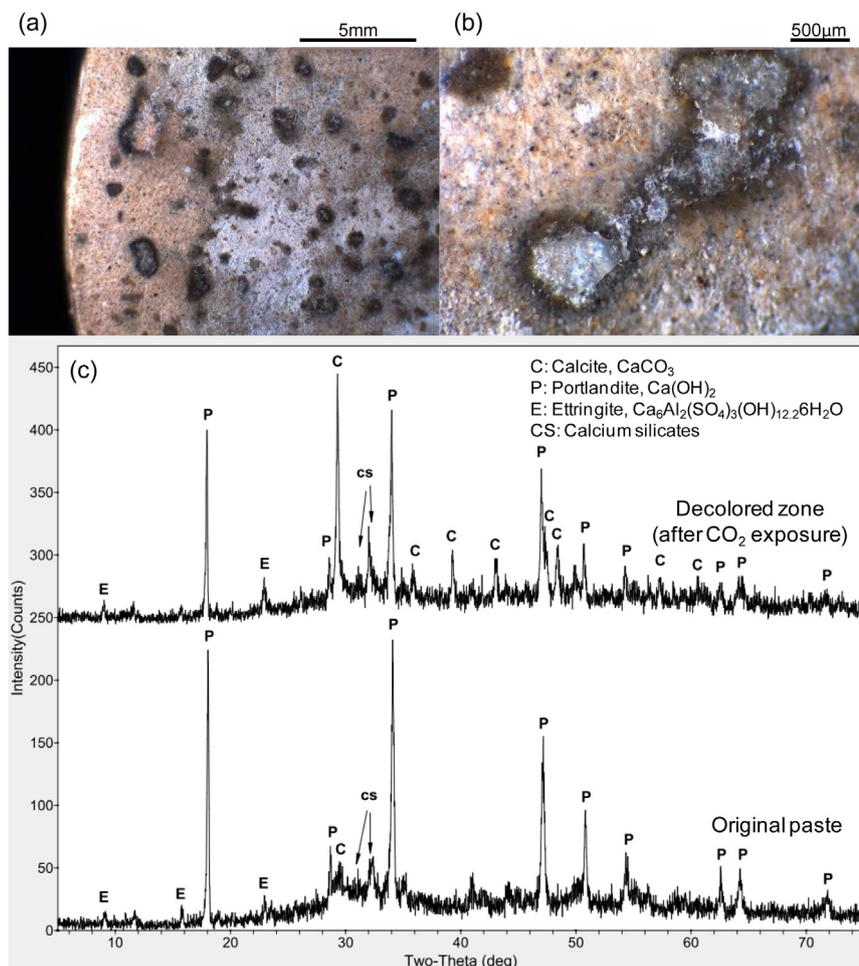
**Fig. 5.** Cement specimens – Post-test forensic analyses. (a) Carbonation on the specimen peripheral surface (orange color). (b) Reaction rim around grains. (c) XRD analysis for the original cement paste and after exposure to  $\text{CO}_2$ . (For interpretation of the references to color in this figure legend, the reader is referred to the web version of this article.)
