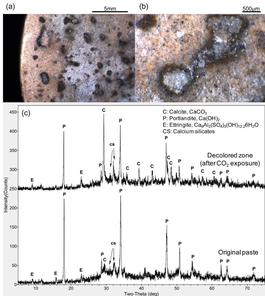
**Fig. 5.** Cement specimens – Post-test forensic analyses. (a) Carbonation on the specimen peripheral surface (orange color). (b) Reaction rim around grains. (c) XRD analysis for the original cement paste and after exposure to CO<sub>2</sub>. (For interpretation of the references to color in this figure legend, the reader is referred to the web version of this article.)
