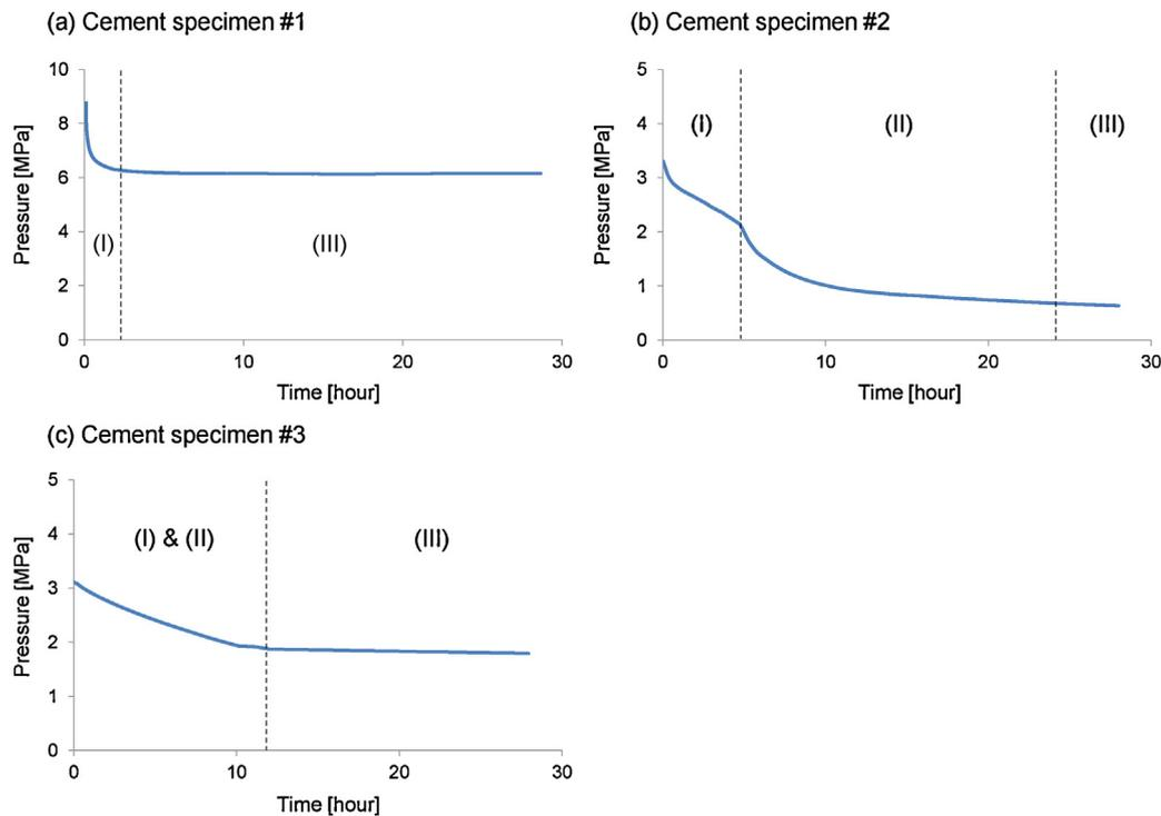
**Fig. 4.** Cement specimens – Shut-off pressures observed with three different specimens. Note: only specimen #2 exhibits a clear transition from single-phase water flow to  $\text{CO}_2$  flow.
