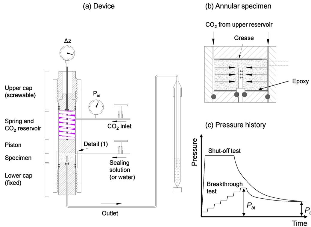
**Fig. 1.** Experimental device for CO<sub>2</sub>-breakthrough and sealing studies. (a) The internal spring applies a constant vertical force onto the specimen. (b) CO<sub>2</sub> infiltrates the specimen radially. (c) Pressure histories typically used for determining breakthrough  $P_{bt}$  and shut-off  $P_d$  pressures in two different test types.
