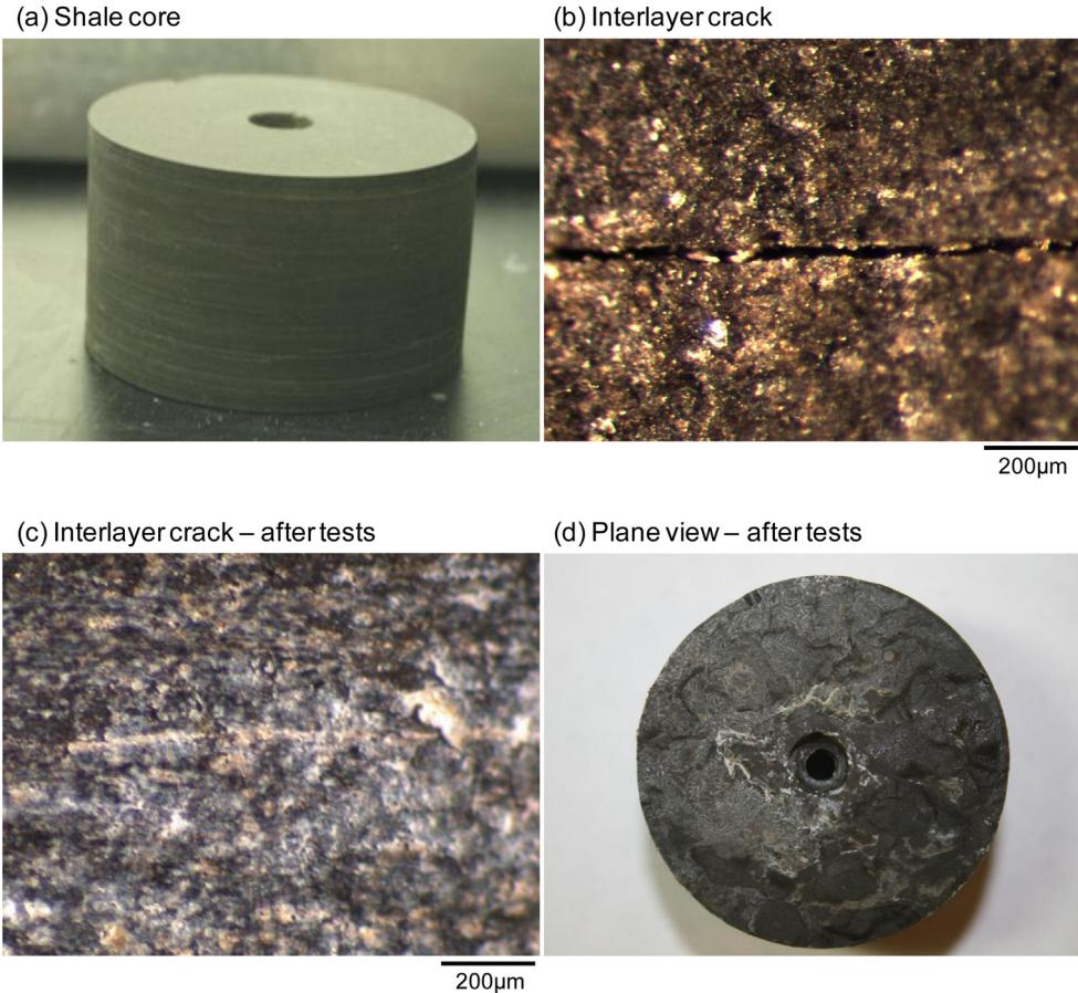
**Fig. 3.** Shale specimens. (a) Core prepared for the CO<sub>2</sub>-breakthrough test. (b) Microscopic image of interlayer crack. Post-test forensic analyses: (c) the microphotograph shows a crack filled with sub-micron bentonite particles after sealing treatments; (d) sub-micron particles deposited in the gap between cracks after sealing treatments.
