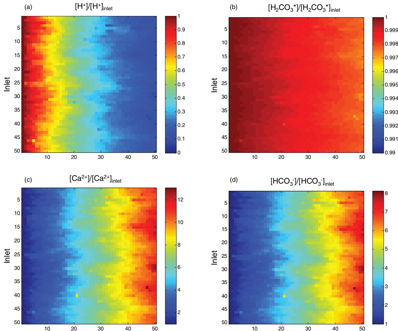
Figure 2. Distribution of species concentration after 1000 network pore volumes have been flushed through the system: (a)  $\text{H}^+$ , (b)  $\text{H}_2\text{CO}_3^*$ , (c)  $\text{Ca}^{2+}$  and (d)  $\text{HCO}_3^-$  ( $i_h = 1000$ ,  $\text{Da} = 1.5 \times 10^{-5}$  and  $\text{Pe} = 6.8 \times 10^3$ ).
