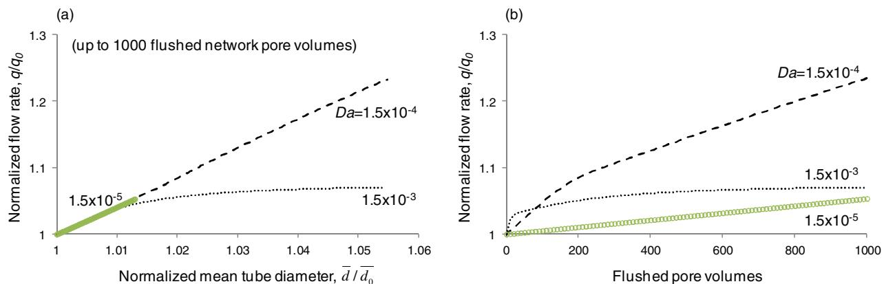
Figure 7. Evolution in flow rate normalized by the original total flow rate  $q/q_0$  with respect to: (a) normalized mean tube diameter  $\bar{d}/\bar{d}_0$ , and (b) flushed pore volume for different Damköhler number  $Da$  ( $COV = 0.4$ ). Note: Damköhler number is  $Da = 1.5 \times 10^{-3}$  for hydraulic gradient  $i_h = 10$ ,  $Da = 1.5 \times 10^{-4}$  for  $i_h = 100$ , and  $Da = 1.5 \times 10^{-5}$  for  $i_h = 1000$ .
