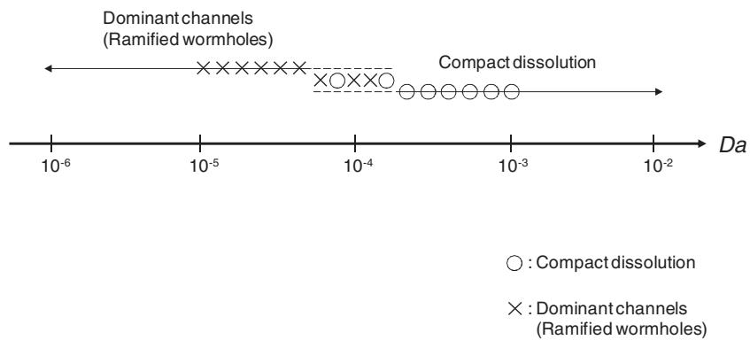
Figure 8. Dissolution pattern as a function of the Damköhler number  $Da$ , for 1000 flushed network pore volumes: CO<sub>2</sub>-dissolved fluid flow through porous media during CO<sub>2</sub> geological storage. Note: network simulations were conducted for various hydraulic gradients  $i_h = 10$  ( $Da = 1.5 \times 10^{-3}$ ), 20-to-200 ( $Da = 3 \times 10^{-4}$ ), and 1000 ( $Da = 1.5 \times 10^{-5}$ ).
