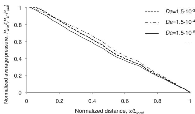
Figure 6. Normalized average pressure at distance  $x$  from the inlet, versus normalized distance  $x/L_{total}$  after 1000 pore volumes have been flushed through the network (Note: in all cases, the initial average pressure distribution is identical to the normalized average pressure shown for  $Da = 1.5 \times 10^{-5}$ ).
