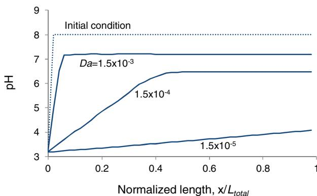
Figure 3. Evolution of pH in space and time: Average pH along the network model after 1000 network pore volumes have been flushed through the system. Note: Damköhler number decreases from  $Da = 1.5 \times 10^{-3}$  to  $Da = 1.5 \times 10^{-4}$  and  $Da = 1.5 \times 10^{-5}$  as hydraulic gradient increases from  $i_h = 10$  to  $i_h = 100$  and  $i_h = 1000$ .
