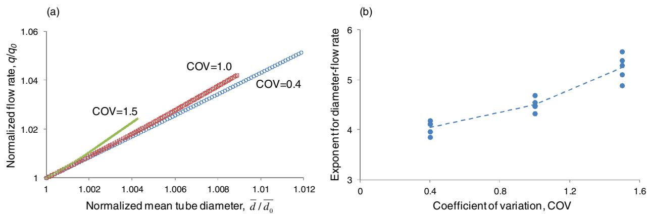
Figure 9. Flow rate and mean tube diameter evolution for different initial coefficient of variations COV in tube diameters. (a) Trends during the first 1000 network pore volumes flushed through the network under a hydraulic gradient  $i_h = 1000$  ( $Da = 1.5 \times 10^{-5}$ ). (b) Exponent  $\alpha$  in  $(q/q_0) = (\bar{d}/\bar{d}_0)^\alpha$  obtained for all simulations.
