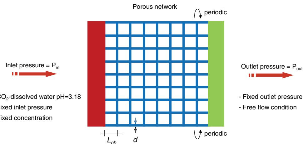
Figure 1. Pore network model: geometry, initial and boundary conditions. Fixed concentration at inlet:  $[H^+] = 6.68 \times 10^{-4}$  mol/L,  $[H_2CO_3^+] = 1$  mol/L,  $[HCO_3^-] = 6.68 \times 10^{-4}$  mol/L,  $[Ca^{2+}] = 1.361 \times 10^{-3}$  mol/L,  $[OH^-] = 1.5 \times 10^{-11}$  mol/L and  $[Cl^-] = 2.72 \times 10^{-3}$  mol/L.
