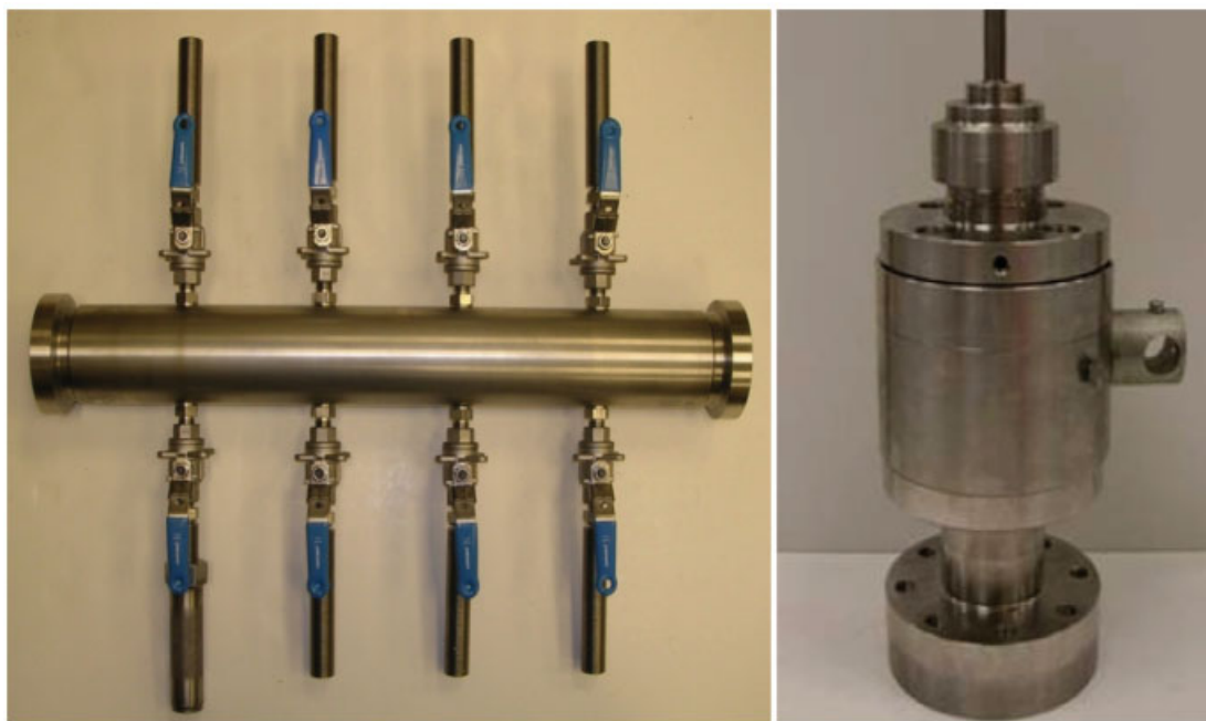
Fig. 7—Pressure-core testing devices developed at Georgia Institute of Technology: (a) instrumented pressure testing chamber (IPTC) and (b) the IPTC- \sigma device permits the application of in-situ state of effective stress to determine effective-stress-dependent properties.
