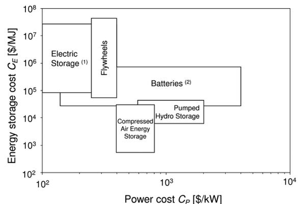
Fig. 4. Energy and Power Costs for Various Energy Storage Systems (Note: (1) Electric storage includes standard electrostatic capacitors, electrochemical capacitors, and superconducting magnetic energy storage; (2) Batteries include conventional, molten salt, lead-acid, and flow batteries (Data from Bradbury, 2010).)
