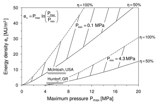
Fig. 2. Energy Density of Compressed Air in Isothermal Conditions (The energy density is a function of the maximum  $P_{max}$  and minimum  $P_{min}$  storage pressures, and the recovery efficiency  $\eta$ . Dotted and continuous lines represent 50 and 100% efficiency, respectively. The energy density of the CAES projects shown was calculated dividing their energy output (total electric energy minus the thermal energy used in the generation stage) by the total volume of the salt caverns.)
