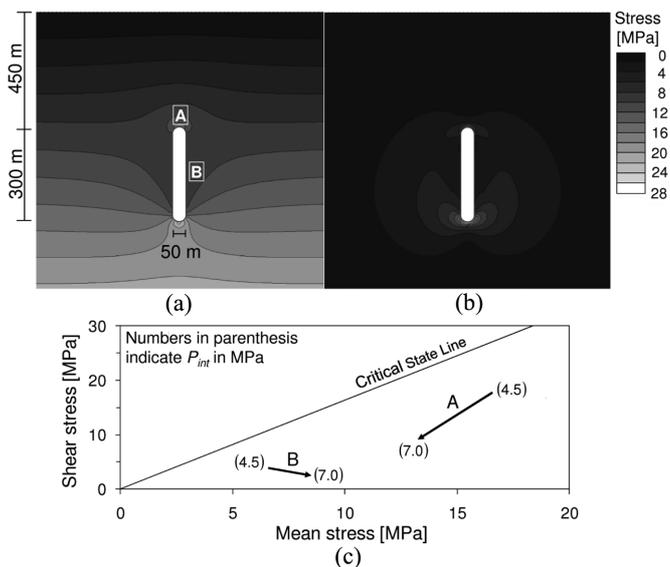
Fig. 6. Underground Cavity in Elastic Medium Subjected to Cyclic Internal Pressure  $P_{int}$  from 4.5 to 7 MPa: (a) Mean Stress, (b) Shear Stress for Internal Pressure of 7 MPa, (c) Stress Paths of Points A and B (Stress field computed using a gravitational stress field and plane strain conditions. Simulated conditions correspond to McIntosh salt cavern.)
