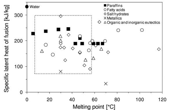
Fig. 1. Possible Phase Change Materials: Melting Point and Latent Heat of Fusion (Data from Sharma *et al.* 2009; and Zalba *et al.* 2003)
