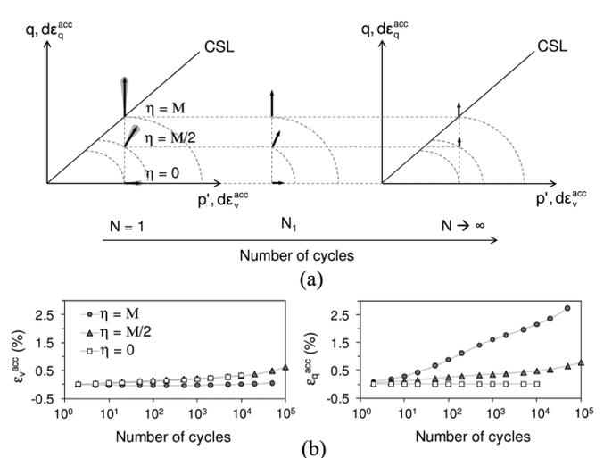
Fig. 7. Cyclic Behavior of Granular Materials: (a) Schematic Representation of the Increments of Volumetric  $\epsilon_v^{acc}$  and Shear Strain  $\epsilon_q^{acc}$  with the Number of Cycles for Soil Elements at Three Different Average State of Stress (The arrows represent the direction and magnitude of the accumulated strain.), (b) Measured Accumulated Volumetric and Shear Strain in Sand with the Number of Cycles for Each Average State of Stress (Data from Wichtmann, 2005)
