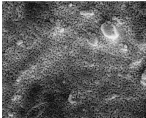
Fig. 1. Specimen 1 (mild rust): SEM photographs of surface features; width of area shown (a) 100 \mu\text{m} ; (b) 10 \mu\text{m}
