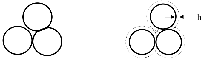
Figure 13. Contact forces and contact deformability - Degradation threshold strain. (a) Large particles: Hertzian deformation. (b) Small particles: electrical interaction.
