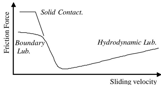
Figure 1 The effect of fluids on friction
