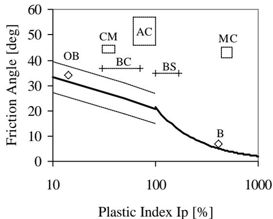
Figure 2 Friction Angle vs Plastic Index - Anomalous soil response. Diamonds: study of organo-clays (see text for details).
