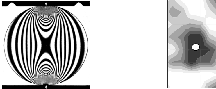
Figure 9. A soil grain \equiv Sensor. (a) Photoelastic disk subjected to a vertical force (Frotch, 1941). (b) Tomographic image of S-wave velocity around a pressured cavity "Stress tomography" (Lee et al. 2005)
