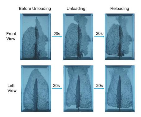
Figure 4. Pressure fluctuations promote the upwards migration of gas-filled openings. Y-shaped gas fracture (Note: unloading from 14 kPa).
