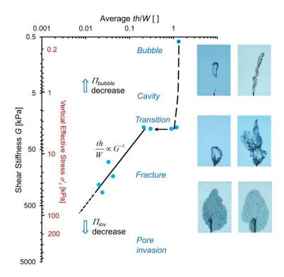
Figure 6. Gas migration patterns in sediments as a function of effective stress and sediment stiffness. The average fracture thickness-to-width ratio th/W is a linear function of sediment compliance  $G^{-1}$ .
