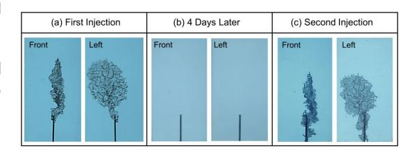
Figure 5. Memory effect. (a) Open-mode gas-filled fracture after the first injection. (b) Gas diffusion and fracture healing 4 days after the first injection. (c) Gas-filled fracture after the second injection.
