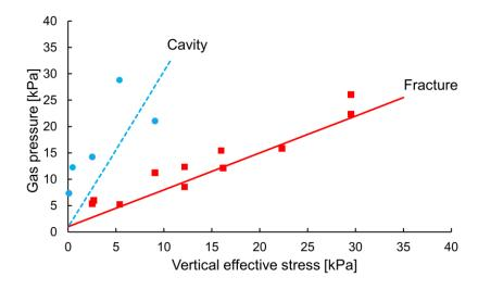
Figure 8. Gas injection pressure vs. vertical effective stress for cavity expansion and open-mode fractures. Data: red squares identify observed fractures; blue circles correspond to cavity expansion (peak pressure). Models: the solid red line is for fracture propagation (Equation 4,  $k_0$ =0.7), and the dashed blue line shows the cavity expansion pressure (Equation 2).
