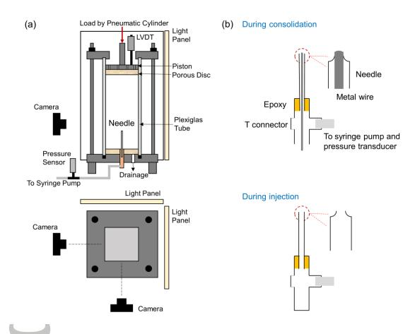
Figure 1. Experimental setup. (a) Frame, cell, and monitoring system - side view and cross section. (b) Details of the gas injection needle.
