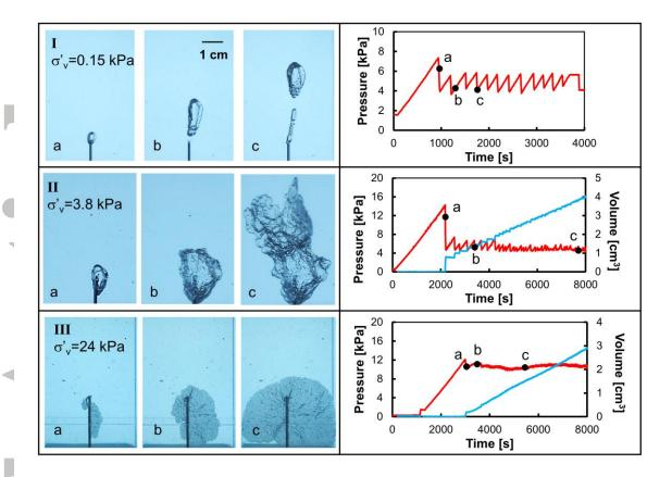
Figure 2. Typical displacive gas migration patterns. Plots on the right show gas pressure (red line) and gas inclusion volume (blue line) signatures.
