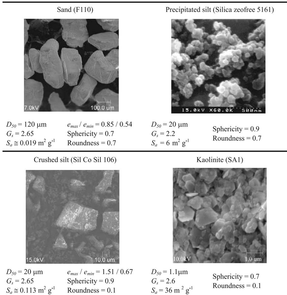
**Figure 1.** Characteristics of tested soils, compiled from *Santamarina and Cho* [2001], *Klein* [1999], *Parks* [1990], and *Guimaraes* [2001]. Specific surface for kaolinite and precipitated silt was measured using methylene blue (wet method). SEM pictures were provided by A. Palomino.
