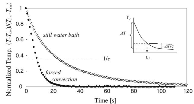
**Fig. 1** Temperature change in a particle ( $r_p = 0.0127\text{ m}$ ) when it is suddenly submerged in a large cold water bath. The insert shows the definition of the characteristic time  $t_{ch}$ . Data shown for cooling in still water and in stirred water
