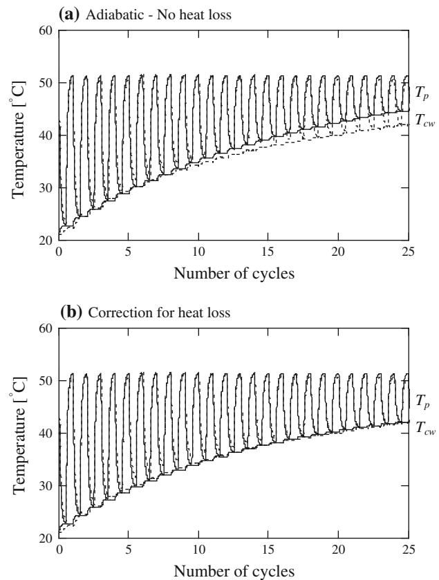
**Fig. 4** Experimental data (dotted lines) and numerical prediction (solid lines) corresponding to the particle and the water bath temperature evolution—Cycle duration  $t_{cy} = 200$  s. Numerical predictions in each frame assume: **a** adiabatic conditions—the overestimated bath temperature increases with time; and **b** heat loss to the surroundings (fitting value:  $\Psi = 0.05\text{W}^{\circ}\text{C}^{-1}$ ). Note:  $T_p$  particle temperature;  $T_{cw}$  cold water bath temperature
