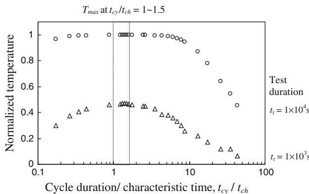
**Fig. 5** Predicted temperature of the water bath at selected times for different cycle durations  $t_{cy}$ . The maximum temperature is obtained when  $t_{cy}/t_{ch}$  is  $1 \sim 1.5$ , where the characteristic time  $t_{ch} = 23$  s. The normalized temperature in y-axis represents  $(T_{predicted} - T_{cw})/(T_{hw} - T_{cw})$
