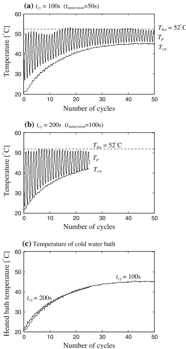
**Fig. 3** Measured heat transfer in two-baths experiments. Temperature evolution with number of cycles for immersion duration  $t_{cy} = 100$  s and 200 s.  $T_p$ : particle temperature.  $T_{hw}$ : constant hot water bath temperature 52°C.  $T_{cw}$ : cold water bath temperature
