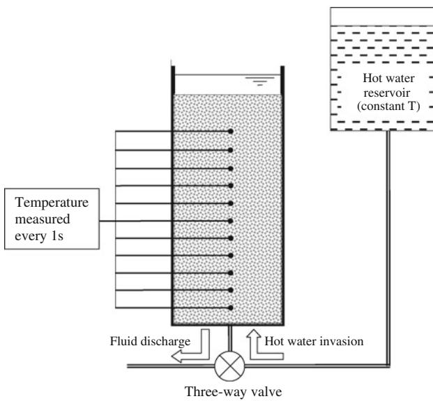
**Fig. 7** Experimental configuration used to study heat transfer during cyclic fluid flow in a granular medium
