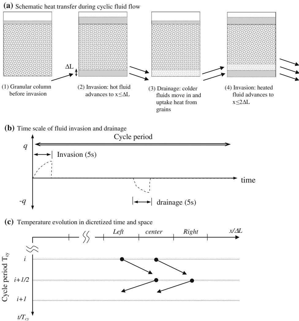
**Fig. 6** **a** Heat transport during cyclic fluid flow. **a-1** A granular column sits on a hot fluid reservoir. **a-2** Hot fluid invades the sediment to height  $x \leq \Delta L$  and transfers heat to grains. **a-3** During the partial drainage phase, colder fluids further away from the boundary  $x > \Delta L$
